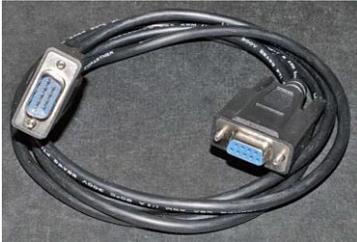
The D-Axe is configured as a data communications device so if connecting to an RS232 interface, a straight-through cable is required. Depending on the RS232 connector the host computer has, this will either be a 9-pin female to 9-pin male, as shown here. Or, in rare instances, you may need a 25-pin female to a 9-pin male cable. In either case, the 9-pin male
