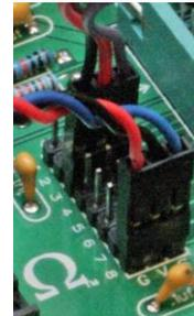
Using this modular approach, proof of concept prototypes can be assembled in mere minutes and the process of writing the code can begin just as quickly. The resulting prototypes are portable, repeatable and robust and not susceptible to damage like a solderless breadboard circuit.
