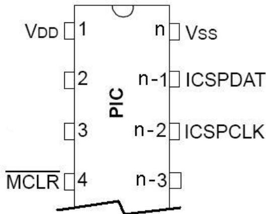
The following is a partial list of PIC microcontrollers that can be used. Check Microchip's datasheets for others.
