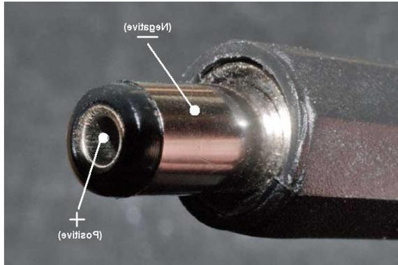
The on-board regulator and standard DC power jack allow for a variety of power options. Any filtered DC source of between 7.5V and 14V can be used. Make sure the chosen power supply delivers positive voltage through the center conductor and negative through the outer sleeve as shown here.
